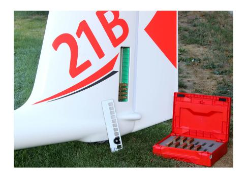
For spin training, spin ballast can be mounted in the fin, see above. Use of spin ballast is only allowed with a payload of max. 242 lbs per seat.
