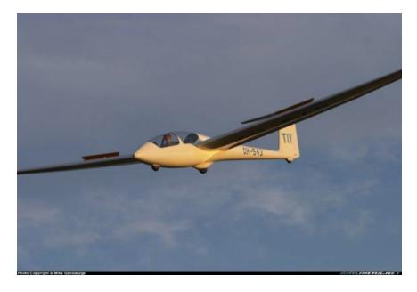
ASK-21 on final approach, before "round-out" or flare to land on main and tailwheel. Use about ¾ Airbrake, 55 knots max. through the "mail slot" at the end of the runway.
