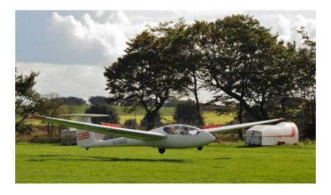
**And this is the Wrong way!** Nose wheel may touch, rebound up, and start the three wheel P.I.O.!
